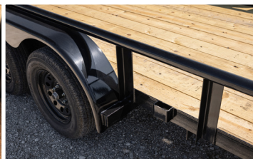
Durable pipe top rail for added strength.
