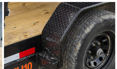
Heavy-duty diamond plate steel fenders are durable and strong.
