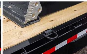
Full-length rubrail & tie down pockets as well as (6) D-rings for optimal cargo control and tie-down options.
