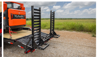
Cleated dovetail and stand-up equipment ramps allow for a low loading angle of equipment.
