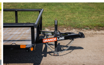
Set-back jack design to prevent tailgate damage on tow vehicle.
